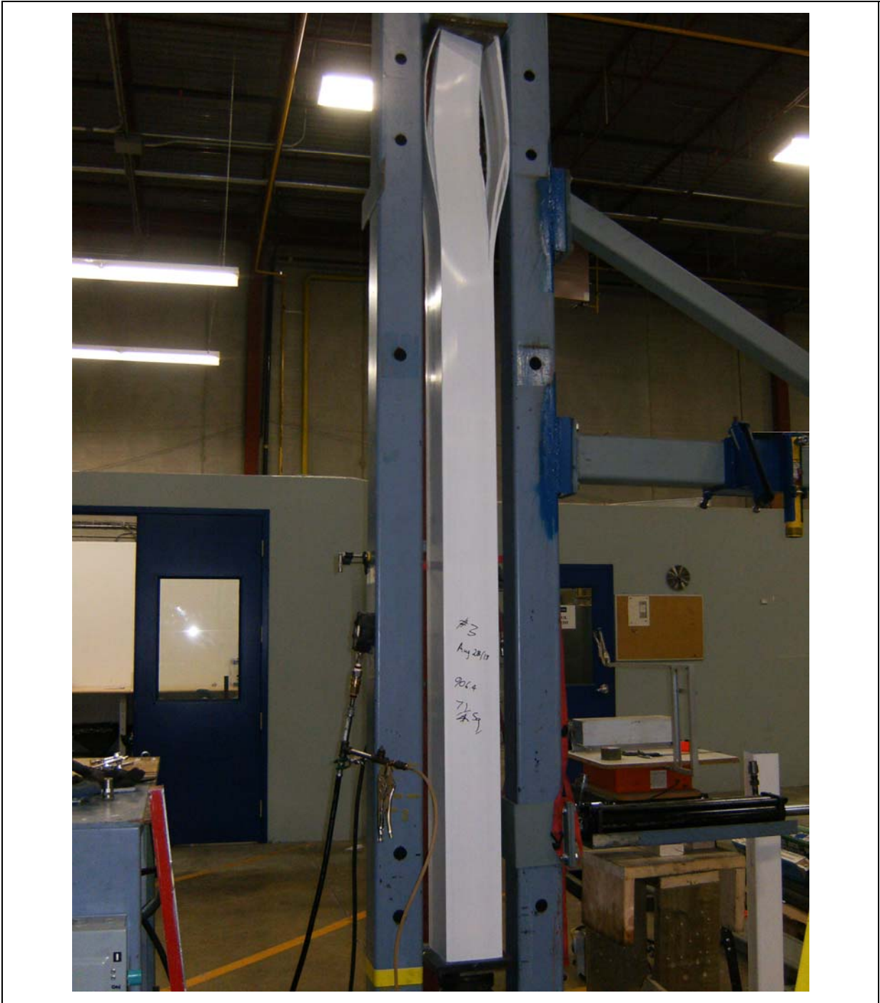
7-1/4 " Square Column Following Fracture
