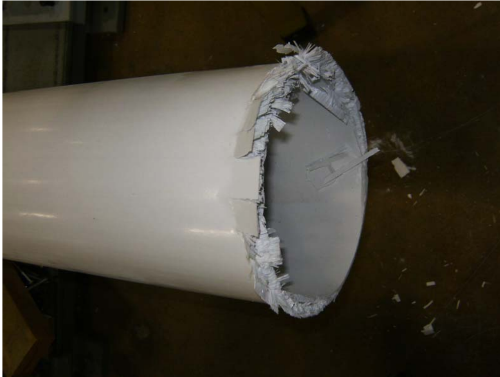
Base of 8" Diameter Round Column Following Fracture
